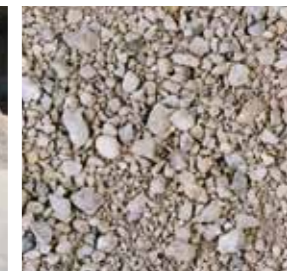
Recycled concrete aggregate
