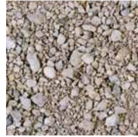
Recycled concrete aggregate
