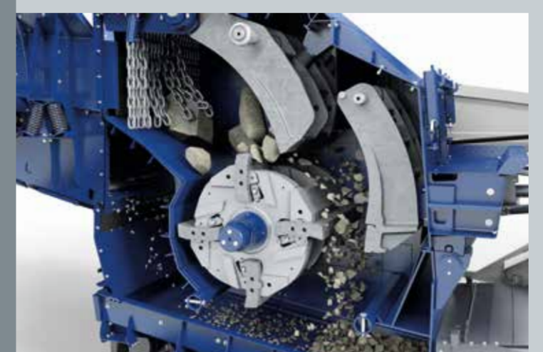
Crusher unit with optimised inlet geometry
