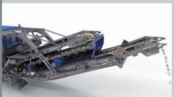
Vibrating screen with extra large screening surface
