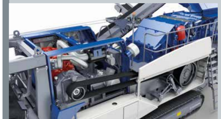
Crusher direct drive via fluid coupling
