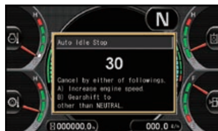
Adjustable idle shutdown automatically turns off the engine after it idles for a set period of time
