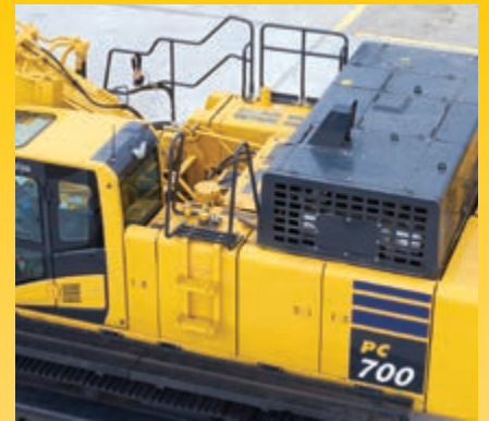
Hand rails and anti-slip plates
