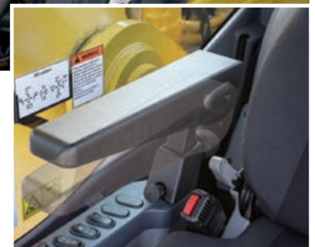
Armrest with simple height adjustment
