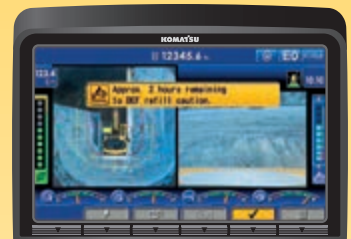
AdBlue® level and refill guidance
