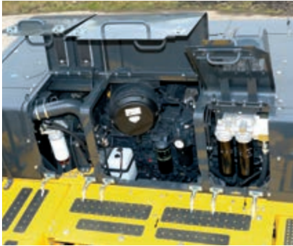
Easy access to filters on the front side of the engine hood
