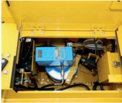
Motorised grease gun equipped with hose reel
