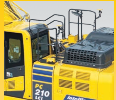
Hand rails and anti-slip plates
