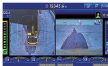
With KomVision, various camera view options help to maintain a constant bird's eye view from above the machine
