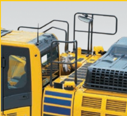
Hand rails and anti-slip plates
