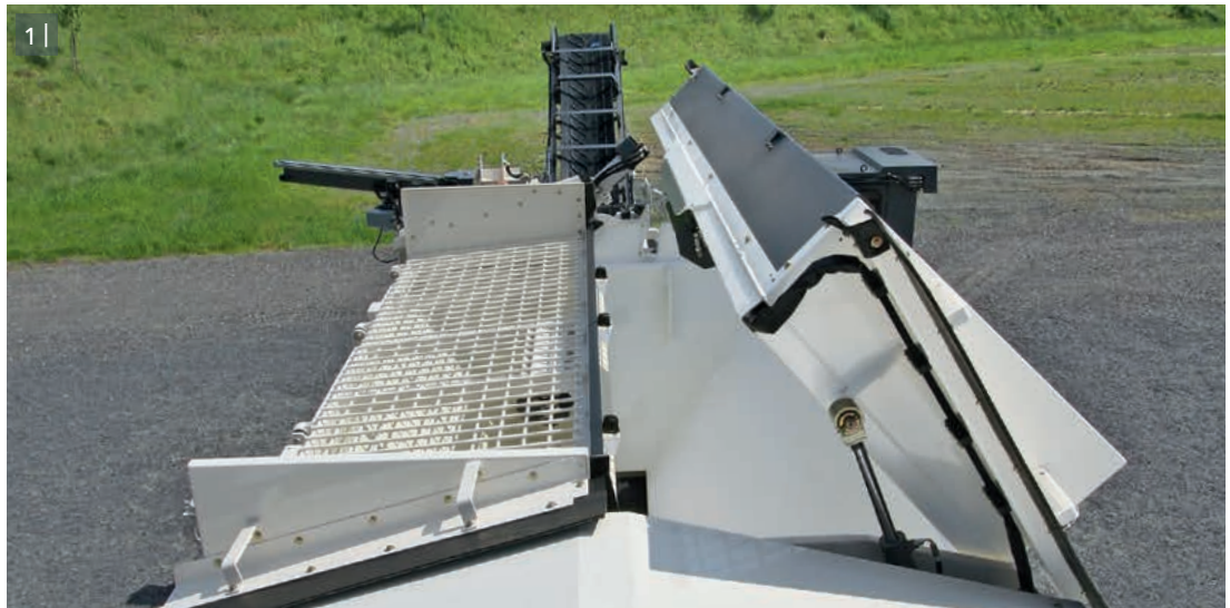
1 | The vibrating screens can also be tilted continuously and independently.
