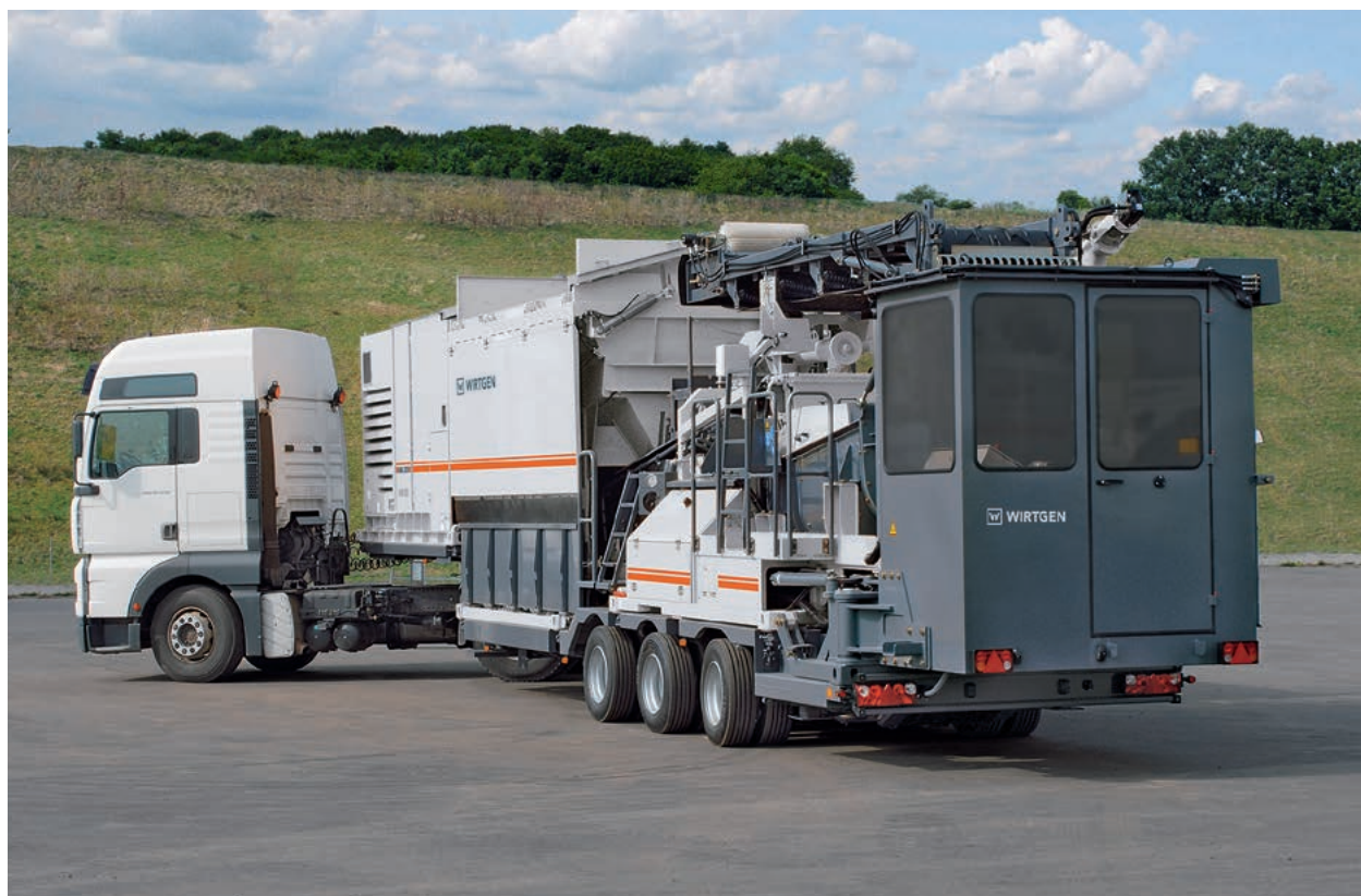
The plant is transported by means of a standard tractor vehicle.
