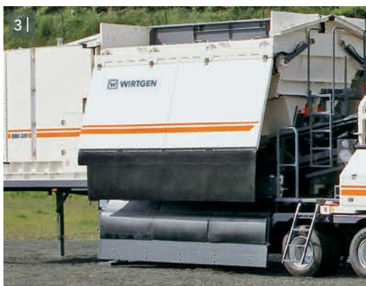
3-4 | Large panels at the sides of the proportioning hopper prevent spilled material from piling up near the plant. Stable panels below the proportioning hopper support the approach ramp.
